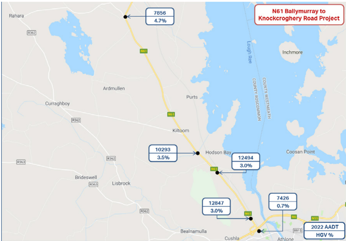
Figure B1.7 2022 AADT and HG% at 19 ATC sites on the N61 Ballymurray to Knockcroghery
